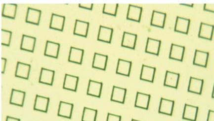
Precise micro structured grid cut out of polymer block
